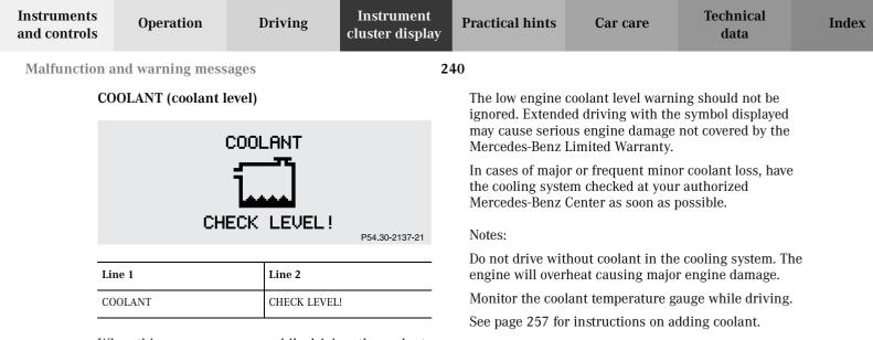
When this message appears while driving, the coolant level has dropped below the required level. If no leaks are noticeable and the engine temperature does not increase, continue to drive to the nearest service station and have coolant added to the coolant system.
